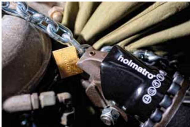
Cutting loose an activist with Holmatro's Special Materials Cutter (see also page 12).
