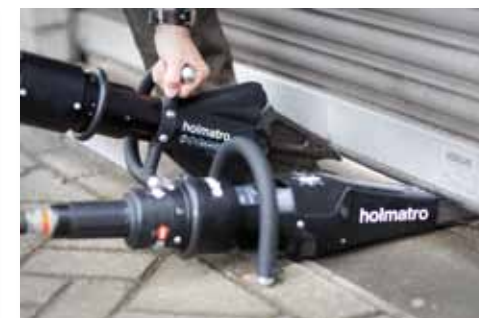
Other equipment, such as a combi tool, can follow up to create a larger opening.
