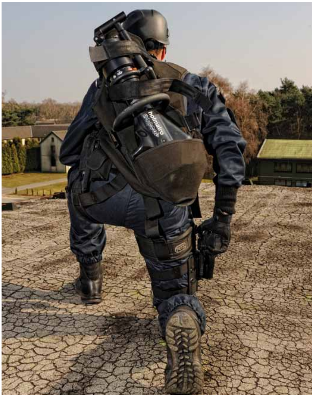
Easy to carry in backpack harness (the same applies to battery-operated tools).
